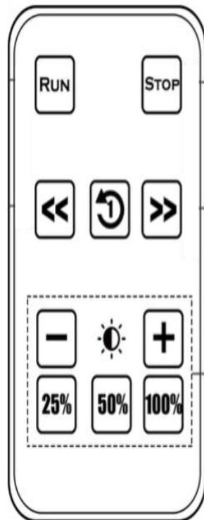
Run: turn the device from 'stand-by' to 'running'
